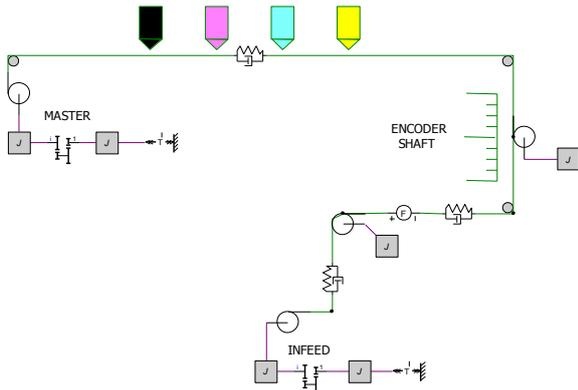
Figure 5 Lumpedmass model of substrate path
